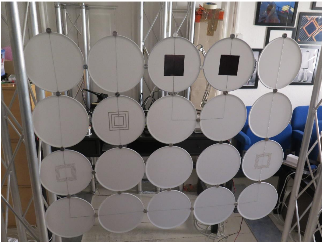
Figure 21: Blind with 1 proximity sensor, two thermochromic discs and two speaker discs
