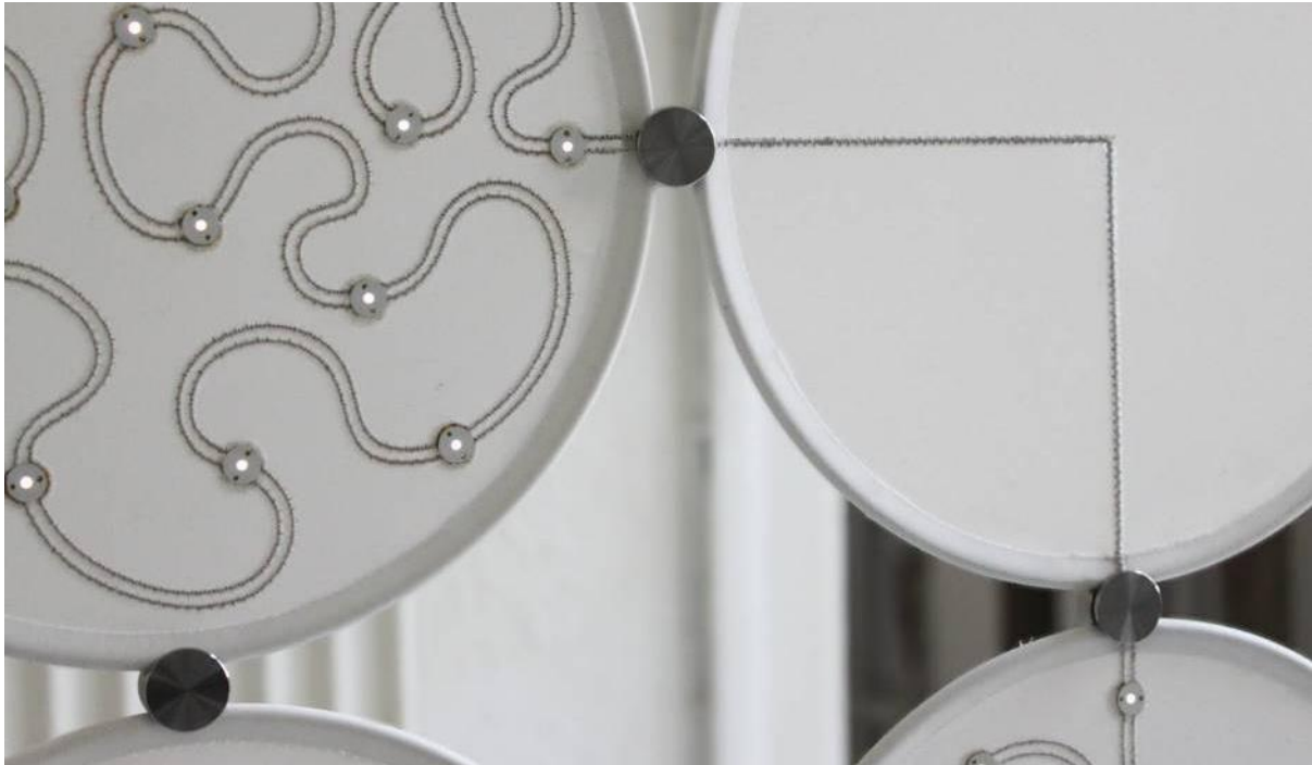
Figure 2: Blind using non-printing technology showing interconnects and light emission
