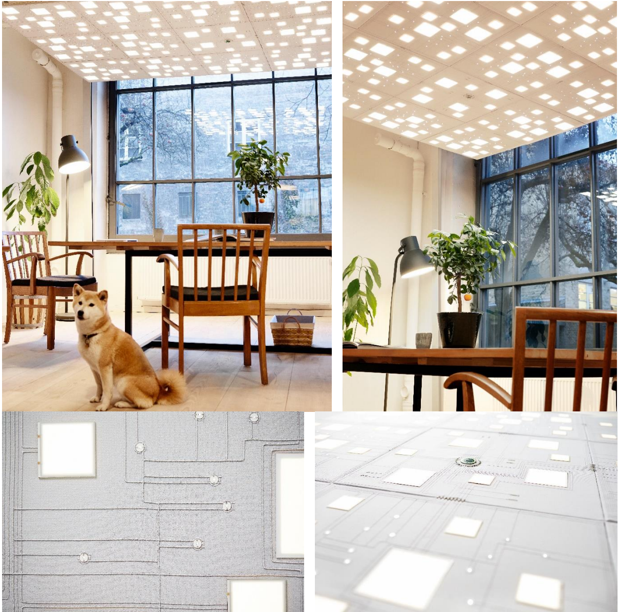
Figure 24: Final ELAC prototype installed in an office (top) and details of the embroidered circuitry (bottom)
