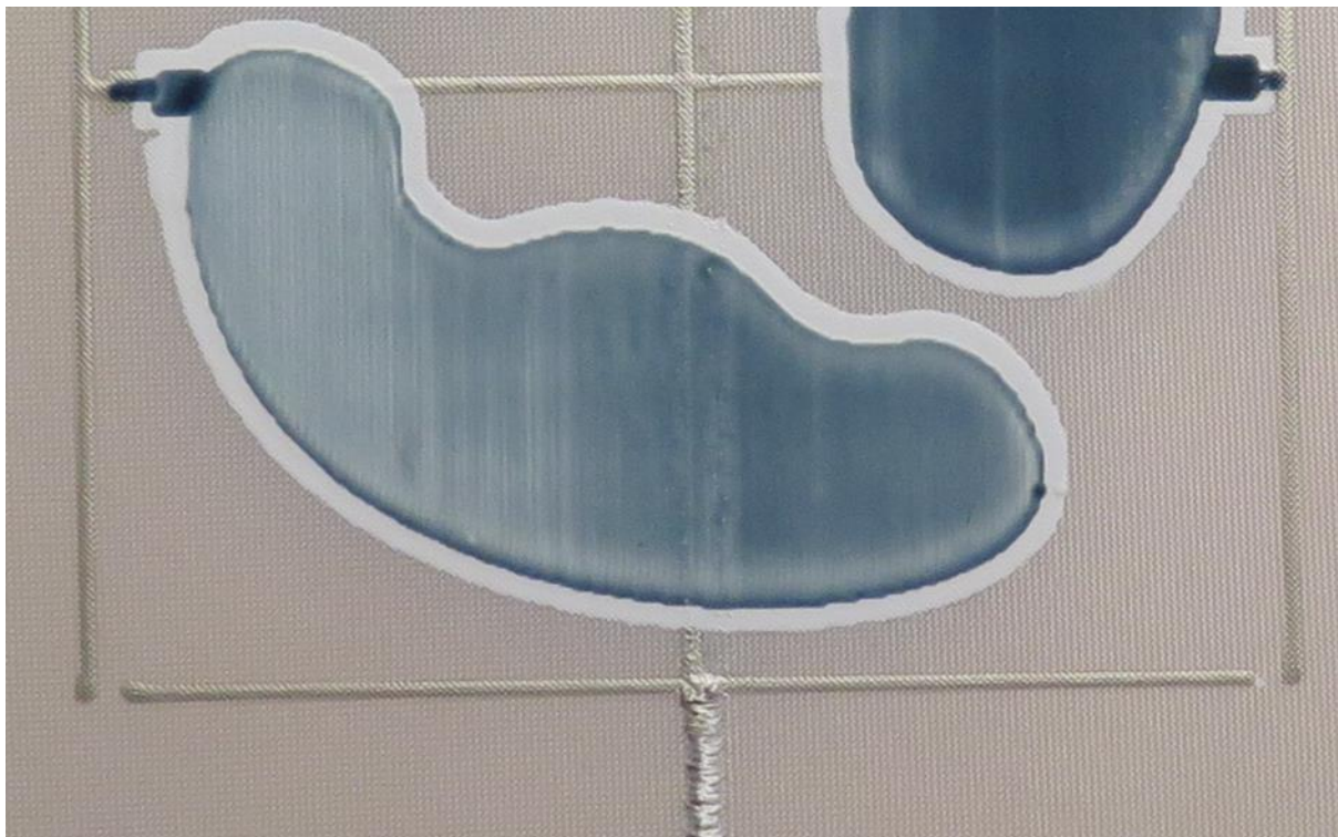
Figure 16: Detail of the EL disc showing the materiality of the light emitting substrate when off.
