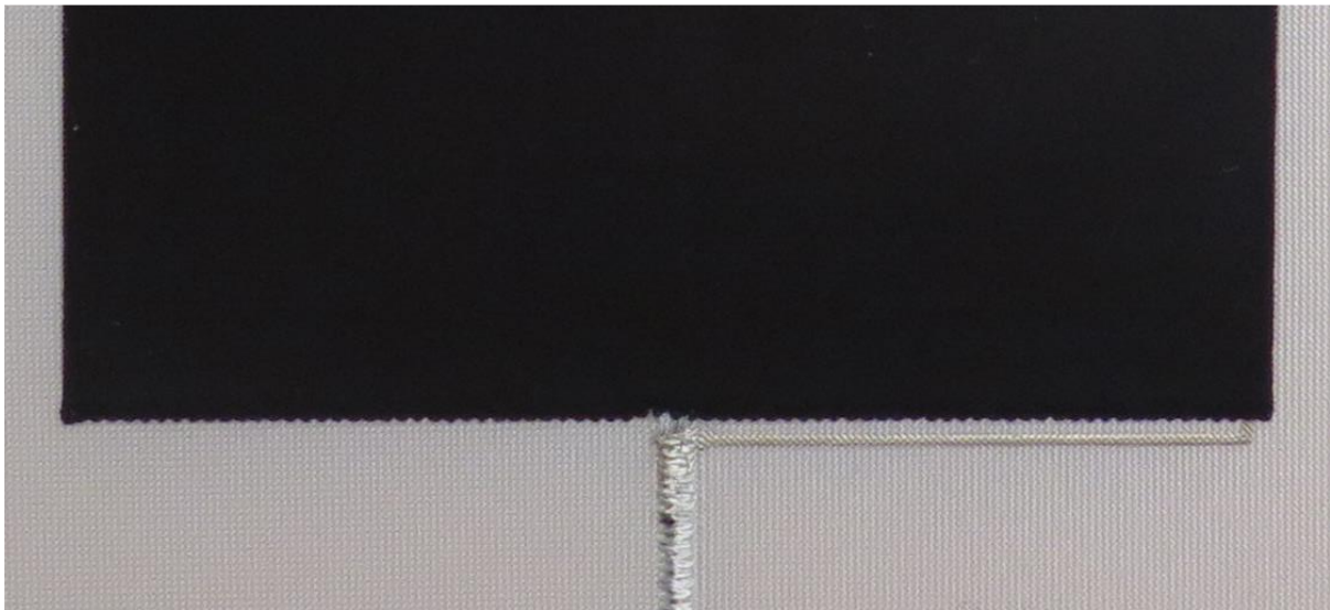
Figure 14: Detail of thermochromic ink showing how the edges differ in the x and y directions.
